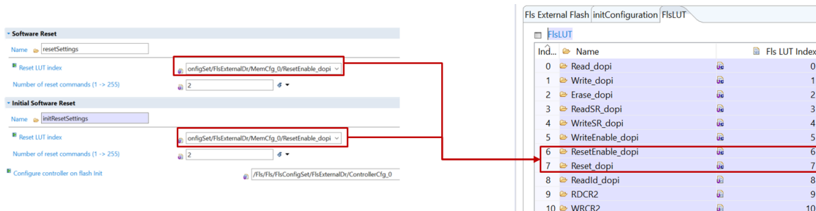
Figure 50. Configure the reset sequence in FLS driver
