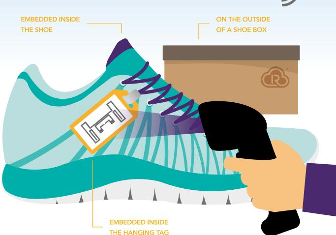
Handheld and wall – or ceiling-mounted readers read the RAIN RFID tags, and can count hundreds of items in a second, even without direct line of sight, so a complete, accurate inventory can be done in just minutes.
